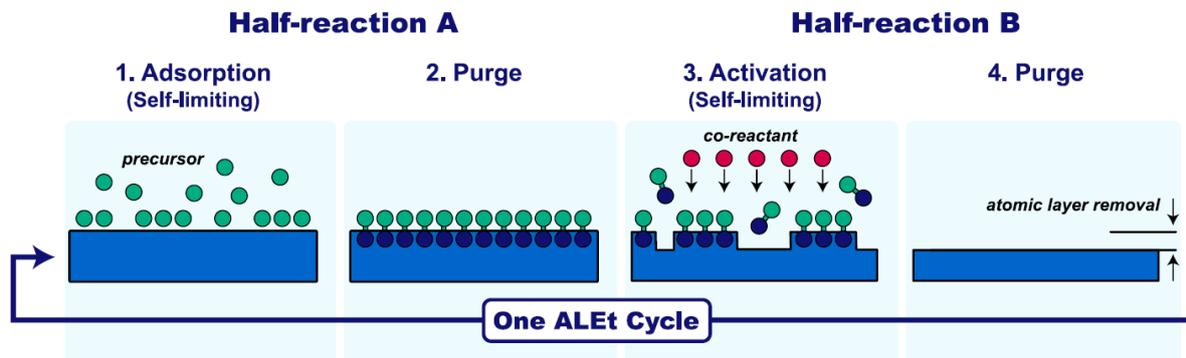
Figure 1: Schematic representation of the chemistry required for atomic layer etching; from Ref 5.
