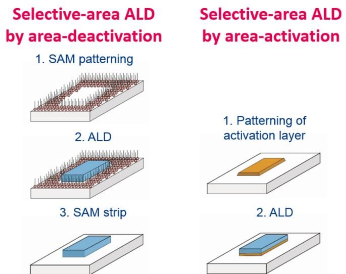
Figure 2: Schematic representation of process flows for two indirect approaches towards selective-area ALD; from Ref 6. By contrast, inherently area-selective ALD (not shown) would exploit the different nucleation chemistry at different substrate areas.
